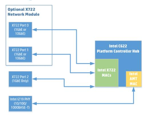
**Note:** When an optional X722 network module is not installed in the system, a "dummy" port is enumerated as Function 0 of the Intel X722 MACs, which allows for the X722 Port 2 on the Motherboard to enumerate.
